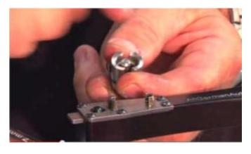
3. Load keepers into tool, one on each side, as it goes on the valve. Let go of clamps
