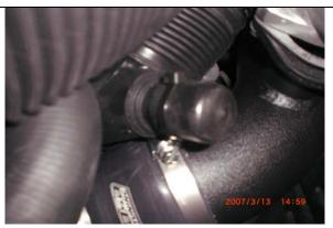
Use rubber caps provided and plug off both holes left by original BOV hoses. Tie strap to secure. These are not under pressure and do not need to be hard clamped.
