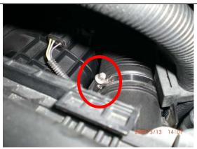
Loosen clamp on accordion hose.
