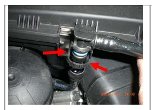
Remove hard plastic line. Squeeze round plastic fitting to release.
