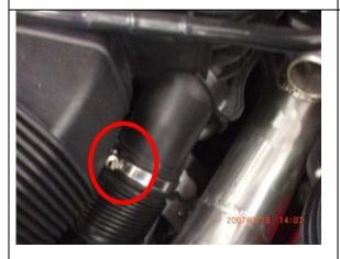
Loosen clamp on front of accordion hose.
