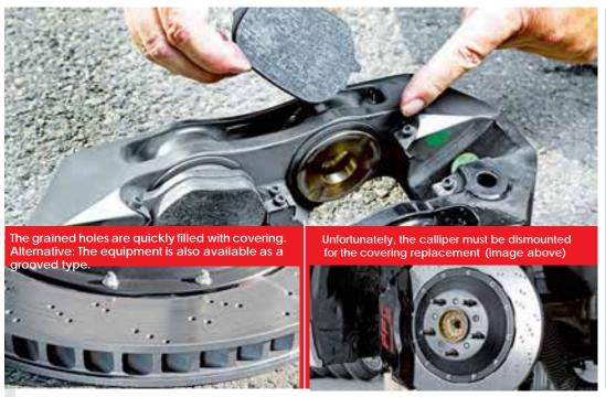
FC - Performance Friction – is primarily known for racing sports. An increasing number of teams rely on these English brakes. To no surprise, since the equipment is the lightest in the test and weighs only 24 kilogrammes. That means about 10
