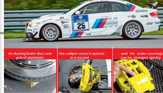
black, red, blue, and silver). On the contrary — the calliper features a cover that can be opened for the easy dismounting of brake coverings. The weight of the equipment is a bit below that of the series, the price of 3,748 euros lies within the usual range. After the initial braking,
