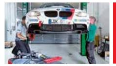
Endurance test: in two days - a DEKRA mechanic and Marc Müller (Lightweight Performance) screwed six brake systems on to the BMW M3. Two hours were sufficient for the replacement of each system. The ventilation was easy and quick for some and lengthier for others. Several litres of brake fluid were required.
